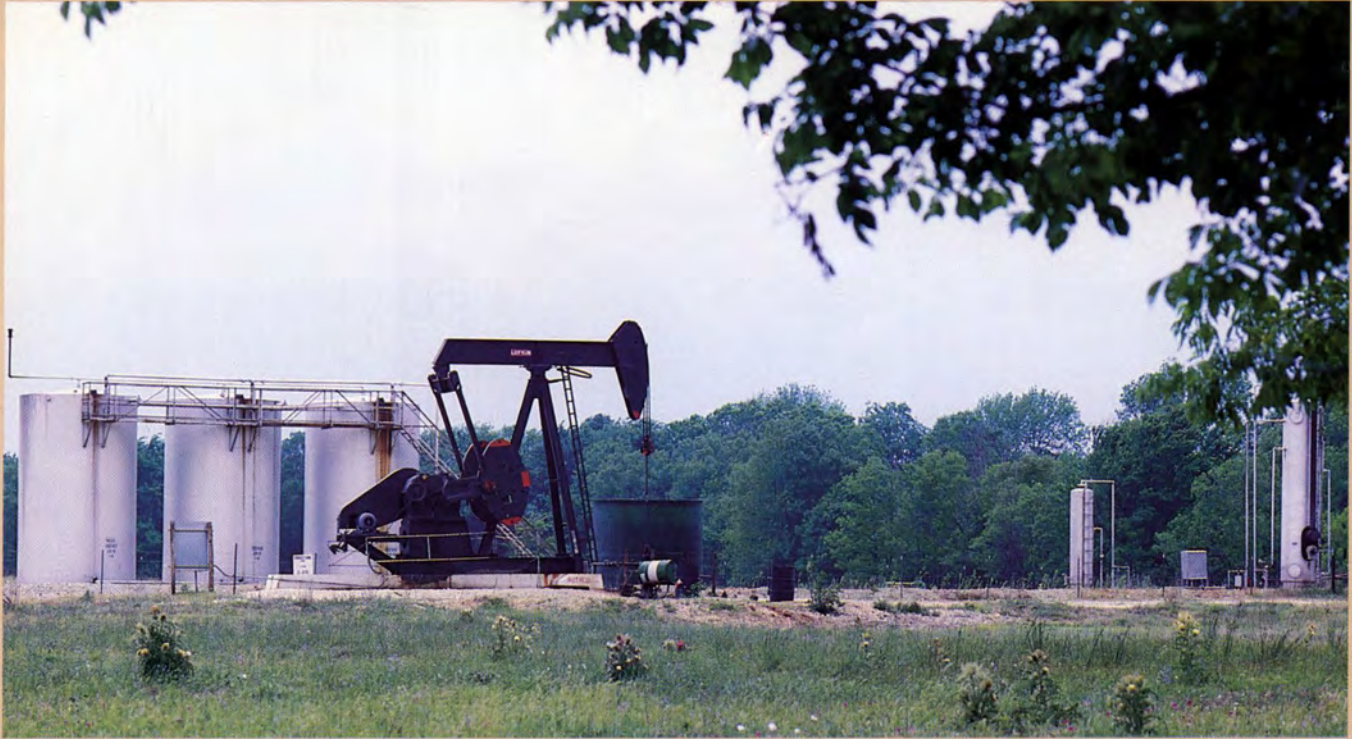
LUFKIN C-228D-213-86 Unit, Lordstone Corporation, College Station, Texas.
