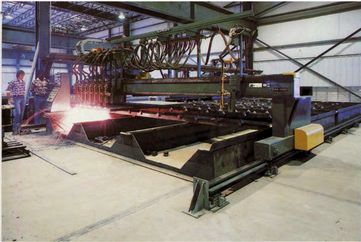
(opposite page, bottom) A special accuracy 120-inch gear hobbing machine combines two operations—gear gashing and finishing—into one single operation. (left) New structural steel facilities house the optimum in welding equipment, including a state-of-the-art torch cutting machine. (below) Automation in the new $7 million structural steel and final shipping and assembly plant has increased productivity and reduced costs.
