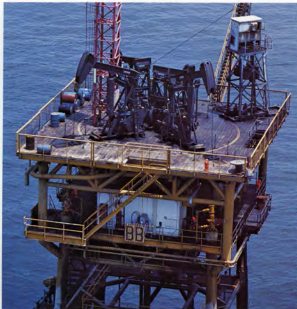
LUFKIN Air-Balanced Units operating on a platform eight miles off the coast of Africa for Elf—Congo, Point Noire, Peoples Republic of Congo
