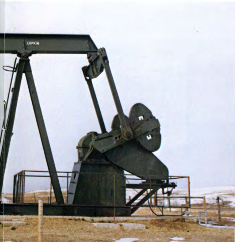
LUFKIN M-320D-256-144 Unit, Canadian Superior Oil, LTD, Harmatten Field, Alberta, Canada
