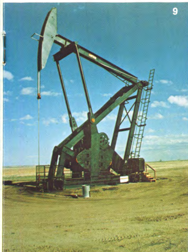
10. LUFKIN C320-305-100 Unit, Anderson Oil Company, Douglas, Wyoming
