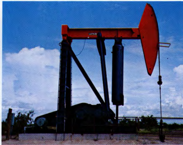
LUFKIN A-640D-168-33.5 Unit, Union Oil Company of California, Odessa, Texas.
