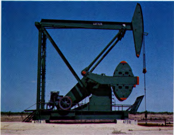
LUFKIN M-640D-305-168 Unit with a LUFKIN 795 CCW Engine, Penwell, Texas.
