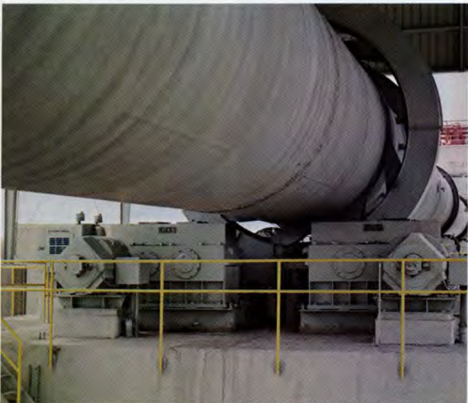
TWO LUFKIN TF-500C reducers drive kiln #4 at Midlothian. Kiln was built by Fuller Company Division of GATX
