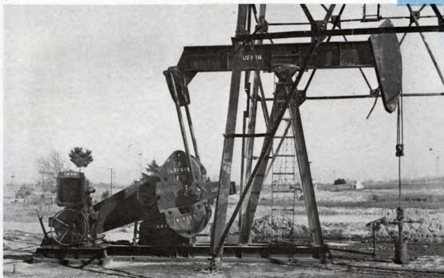
6. Lufkin TC-33A-18B unit with GSC Cooper-Bessemer engine; S. H. Killingsworth; Norman Paul field in Wood County near Quitman, Texas.
