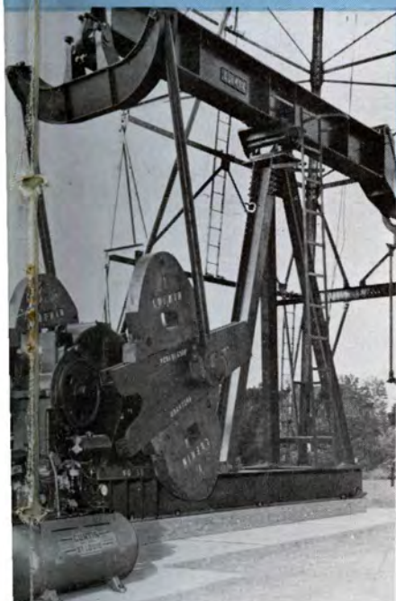
6. GSD-H Cooper Bessemer engine; Field near Pittsburg, Texas.
