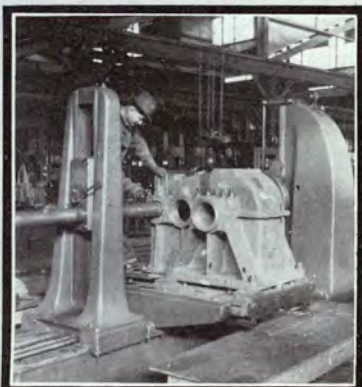
MODERN BORING BARS INSURE ABSOLUTE BEARING ALIGNMENT
