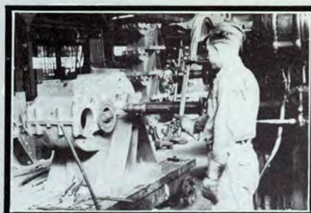
HORIZONTAL DRILLING TO JIG AND TEMPLATE
