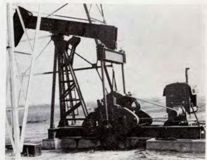
Atlantic Oil Producing Company, Rolf No. 3, Lorraine, Kansas, Lufkin No. TC 2-26 Unit with YT 381 Buda engine.
