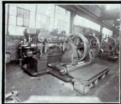
GENERATING LUFKIN SYKES HERRINGBONE GEARS
