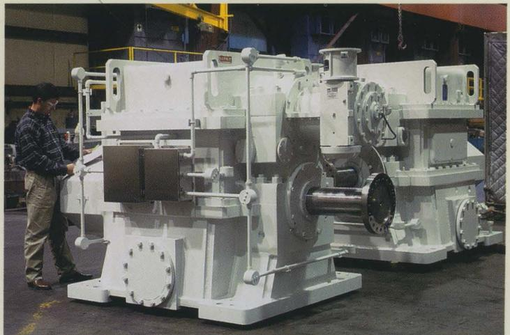
*Gas Turbine Generator Drive for the Power Generation Industry*
