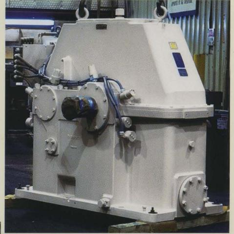
*Centrifugal Compressor Drive for the Petrochemical Industry*
