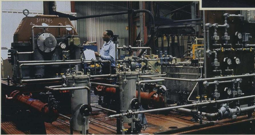
*This Customized Lubricating System is Designed to Furnish Oil to Both the Gear Unit and Customer Equipment*
