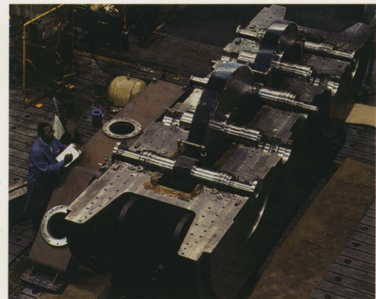
During production, a Lufkin Model CVC804L is inspected by a Lufkin engineer to ensure optimum accuracy and operating performance.
