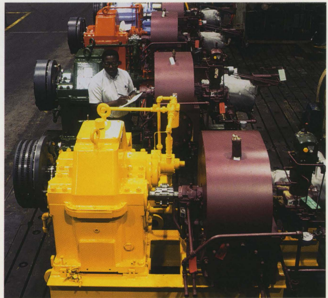
Lufkin is a major supplier of high-speed reducers for sugar mill service, shown here with disengaging clutches.
