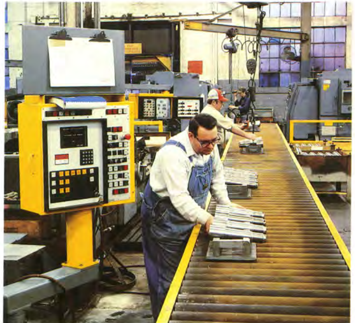
A crank pin production line operates in the Shaft Shop
