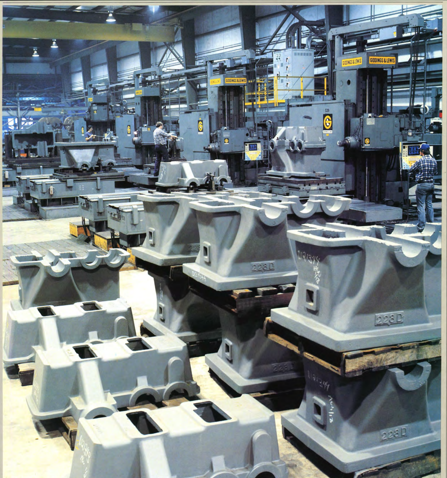
These numerically-controlled machining centers complete many operations at one location
