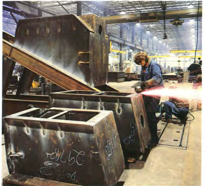
Grinder works at pumping unit sub-base assembly station
