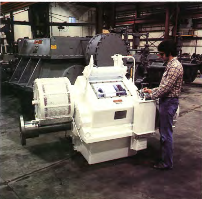
New marine gear has higher horsepower, quiet operation in smaller package. Gears are case-hardened and ground
