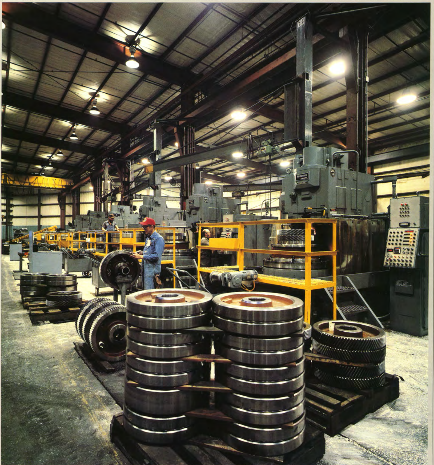
These gear shaper machines cut production time, thereby reducing costs on pumping unit gears
