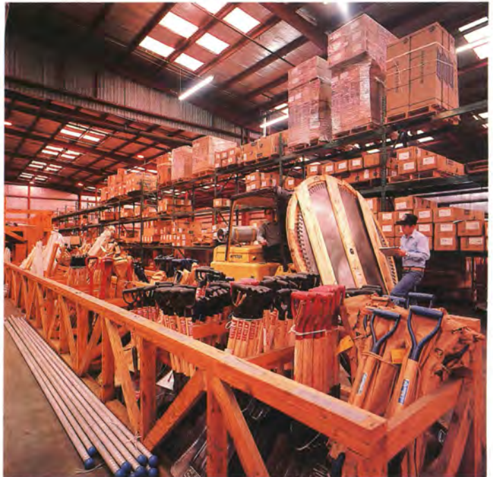
Saws of various sizes are stocked. This saw is 84 inches in diameter and is used in the timber industry
