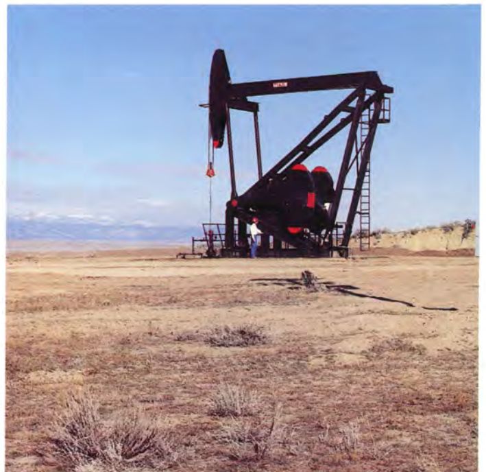
The world's deepest rod pumped well is produced by a Mark II pumping unit in Wyoming from 14,500 feet
