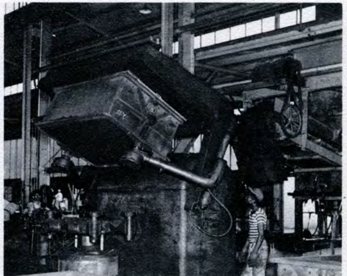
Large moulding machine. Capacity 12,000 pounds.
